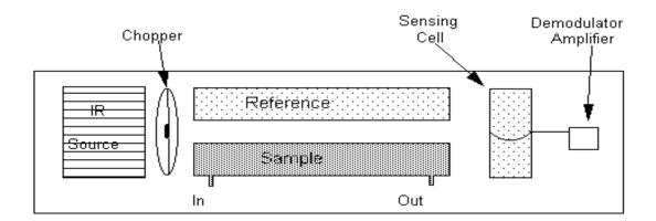
❖ The sample cell contains the compounds to be analyzed, whereas this compound is not present in the reference cell. The reference cell is usually filled with an inert gas, usually nitrogen.
