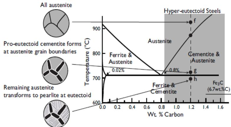
The cooling of a hyper-eutectoid steel is depicted in the above figure with a composition of 1.2 wt.% C from the austenite phase field (point f).
